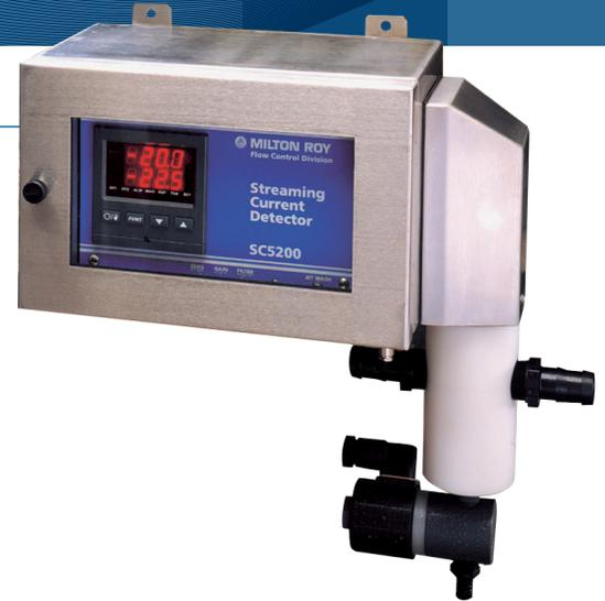
The SC5200 is a complete SCD and process controller in one package. Once installed, it is ready to control any coagulant dosing pump or control valve that accepts a 4-20 mA process signal. No other control instruments are required for a closed loop control.
