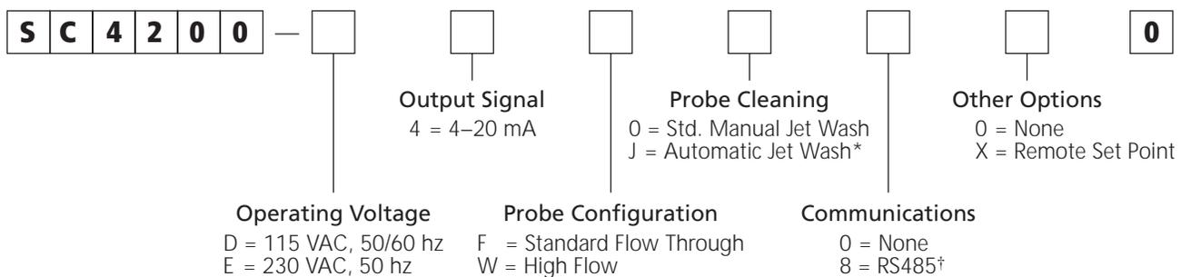
\* Automatic Jet Wash is factory set at 30 seconds every 2 hours. Jet Wash timing is field adjustable. Available settings are 30 seconds to 7 minutes (30 second intervals) every 15, 30, or 45 minutes or 1, 2, or 4 hours.
