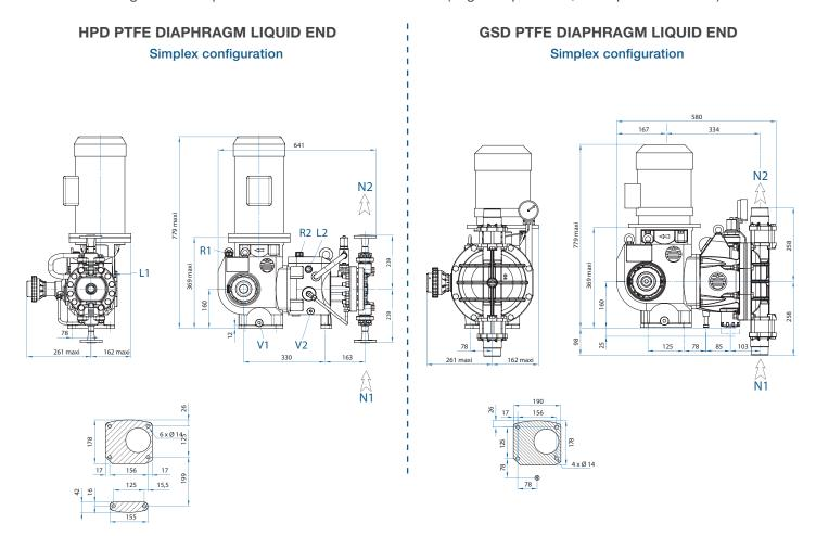
N1 Suction - N2 Discharge - V2 Drain hydraulic oil - L2 Hydraulic oil level - R2 Hydraulic oil filling - V1 Drain mechanic oil - R1 Mechanic oil filling - L1 Mechanic oil level
