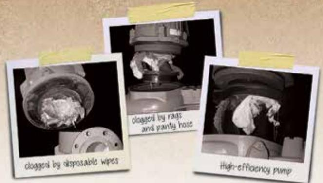
*In rigorous clog testing, Barnes SH clog-resistant pumps outperforms the competition.*
